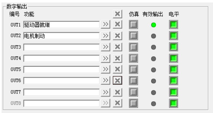
OUT2 外接继电器驱动电机抱闸
