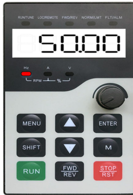
Figure 4-6 Frequency converter power-on display
