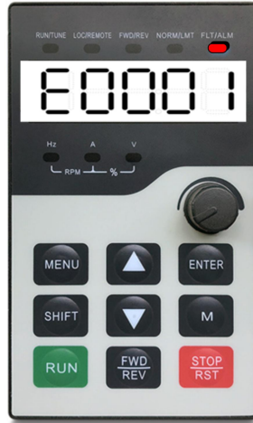
Figure 6-1 Interface fault display
