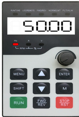
Figure 4-6 Frequency converter power-on display
