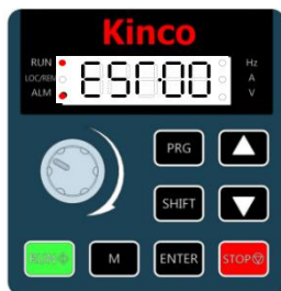
Figure 5-30 Self learning mode operation panel
