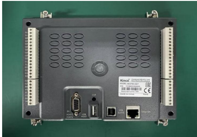
Figure 3.3-4 Install the fixed accessories on the upper and lower sides
