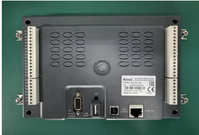
Figure 3.3-5 Install the fixed accessories on the left and right sides
