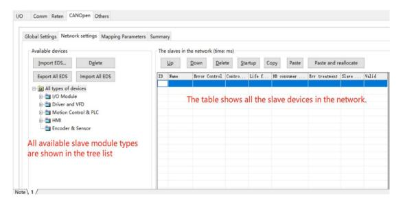
All function buttons on the page have corresponding right-click menu commands. When the user clicks the right mouse button at the relevant position, the corresponding right-click menu will pop up, and the menu command can be used at this time. The following describes the common process of configuring a slave.
