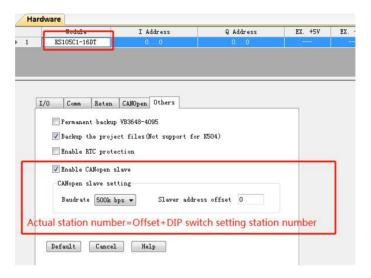
[Enable CANOPEN slave]: If this option is selected, this PLC will act as a CANOpen slave. [Baud rate]: Select the baud rate used by the CAN interface. The baud rate of all nodes in a network must be consistent.
