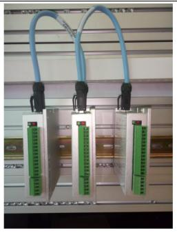
We don't need to setup address for connecting expansion modules. The real address in the net depend on the turn that KincoBuilder configurate hardware.
