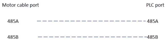
Figure 3-5 485 communication wiring diagram
