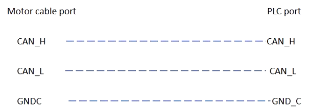
Figure 3-6 CAN communication pins and wiring diagram
