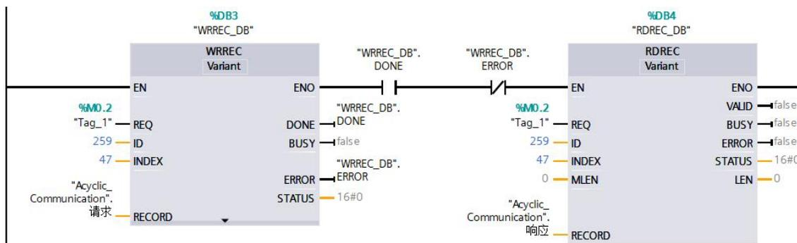
3. The following utilizes the WRREC / RDREC block to read/write CMD\_q\_Max [607300]. The parameter index is 0x6073, subindex is 0x00, and data type is uint16, so the sending command word for writing parameter is 0x2B, and for reading parameter is uniformly 0x40.
