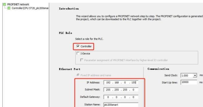
4. Add the servo to the device table, set the IP address and device name (need to be the same as the actual connected device), and then click "Next" :
