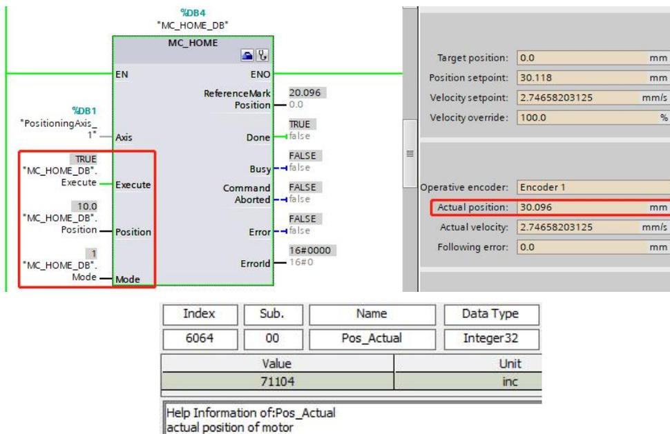
After the homing motion is completed, no matter what position the axis moves to, as long as the PLC is powered off, the actual position data of the axis will be lost and become 0, instead of being converted over with the current encoder value of the drive.
