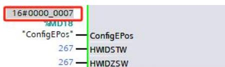
Activate the software limit function, set the soft positive limit [607D01] and the soft negative limit [607D02] for the drive.
