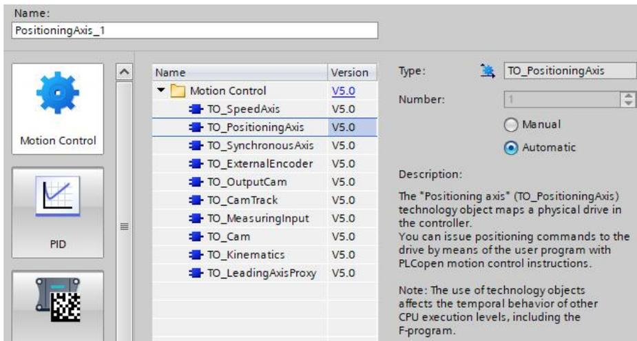
11. Click "Technology objects → PositioningAxis\_1 → Configuration → Basic parameters", select Axis type:
