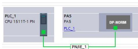
4. If PLC is required to automatically configure the device name of drive (the premise of automatic allocation is that the name of the drive is empty), the topology diagram must be connected. In the topology view, connect the ports according to the actual situation.
