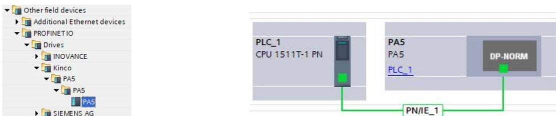
3. If PLC is required to automatically configure the device name of drive (the premise of automatic allocation is that the name of the drive is empty), the topology diagram must be connected. In the topology view, connect the ports according to the actual situation.
