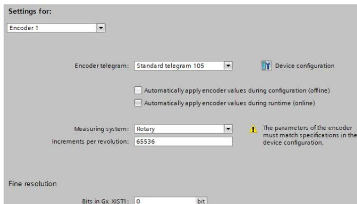
If a Kinco multi-turn absolute encoder motor is used, the Increments per revolution is Feedback\_Resolution [641003], e.g. 65536, and the Number of revolutions is also set to 65536, with Fine resolution selections G1\_XIST1 bit 0 and G1\_XIST2 bit 0:
