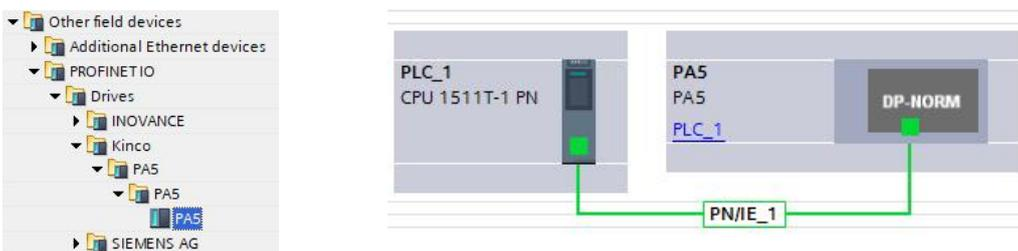
4. If PLC is required to automatically configure the device name of drive (the premise of automatic allocation is that the name of the drive is empty), the topology diagram must be connected. In the topology view, connect the ports according to the actual situation.
