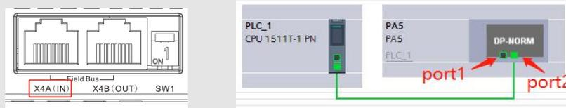
4. Double-click the PA5 module, click "Ethernet addresses" in "General", and set the configured IP address and PROFINET device name. The device names need to be consistent with the actual device names of the drives. When there are multiple drives, the device names cannot be the same:
