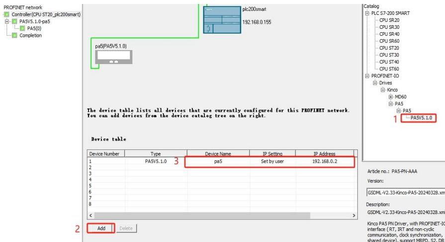
5. Add the PROFIdrive module for the servo, and the submodule of Standard Telegram 3 will be added by default. If only acyclic communication is carried out, the submodule of the telegram can be deleted:
