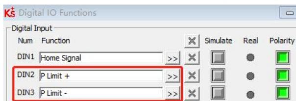
Please note that only positive and negative limits are configured in the KincoServo+ software, but bit 3 of "ConfigEPos" is not set to 1, then the hardware limit function will not take effect.
