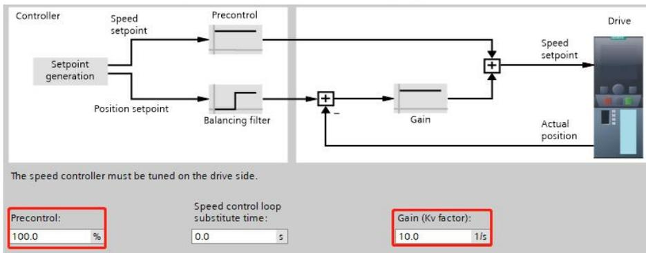
In the above figure, "Gain (Kv factor)" can not be 0, its specific value will not affect the servo's position loop proportional gain, keep it as the default value; "Pre-control" is the percentage of speed feedforward, and the role of K\_Velocity\_FF [60FB02] is the same:
