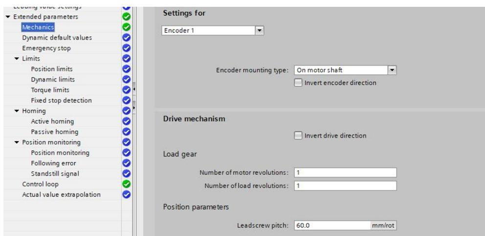
17. Click "Extended parameters → Position monitoring → Following error" to disable the following error monitoring. When monitoring is enabled and the following error setting is small, the PLC will report error easily after enabling operation:
