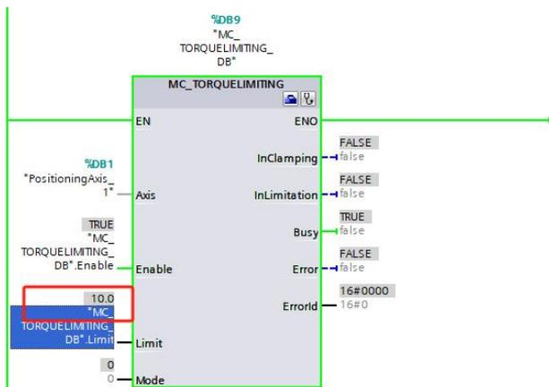
3. When I\_q [607800] reaches CMD\_q\_Max [607300], the output pin "InLimitation" is set to 1, and the drive message status word MELDW's bit 1 is set to 0 (see Table 1-19).
