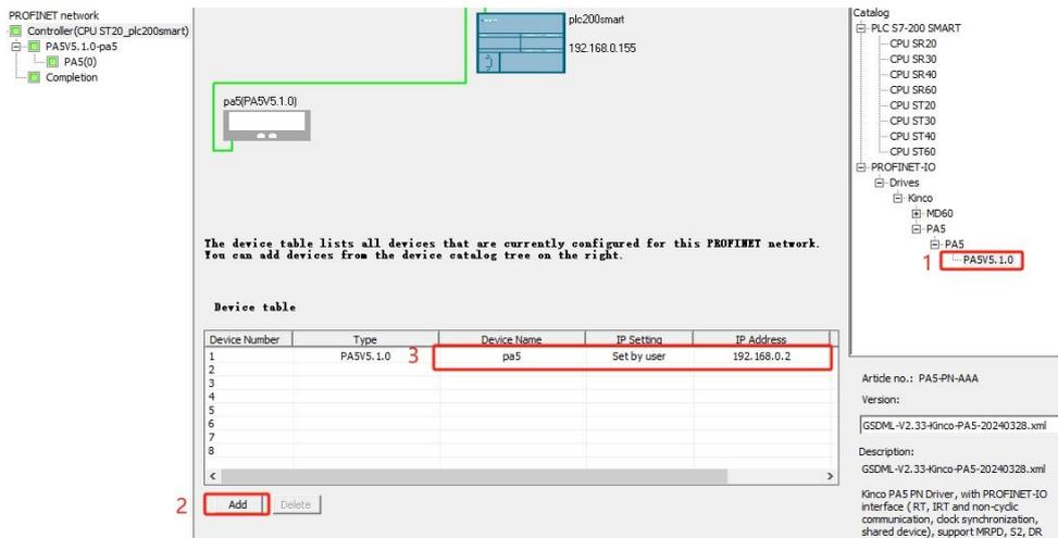
5. Add the PROFIdrive module to the servo, then select and delete the submodule of standard telegram 3 added by default, add the submodule of standard telegram 111, and note down the start address of the I/O data which is needed when calling SINA\_POS:
