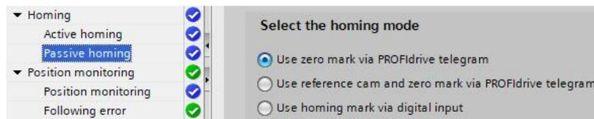
1. Use zero mark via PROFIdrive telegram (i.e. detecting zero mark)
