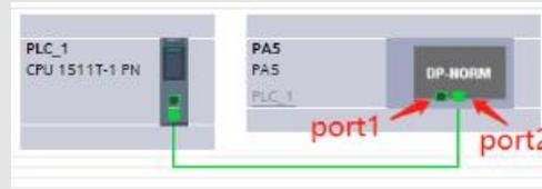
5. Double-click the PA5 module, click "Ethernet addresses" in "General", and set the configured IP address and PROFINET device name. The device names need to be consistent with the actual device names of the drives. When there are multiple drives, the device names cannot be the same:
