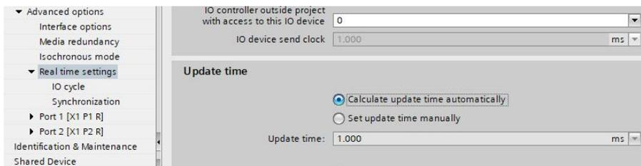
The update time of the configuration needs to be consistent with the ECAN\_Sync\_Cycle [301101], set to 0 for 1ms:
