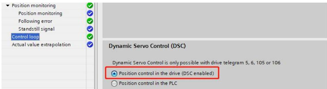
20. After the technology object has been configured, click "Program blocks → MC-Servo [OB91]" in the drop-down list of PLC\_1 on the left side, and then right-click to open the properties to set the PLC application cycle. Please note that when using the DSC function, the PLC application cycle, device update cycle (see Article 8) and ECAN\_Sync\_Cycle [301101] must be the same.
