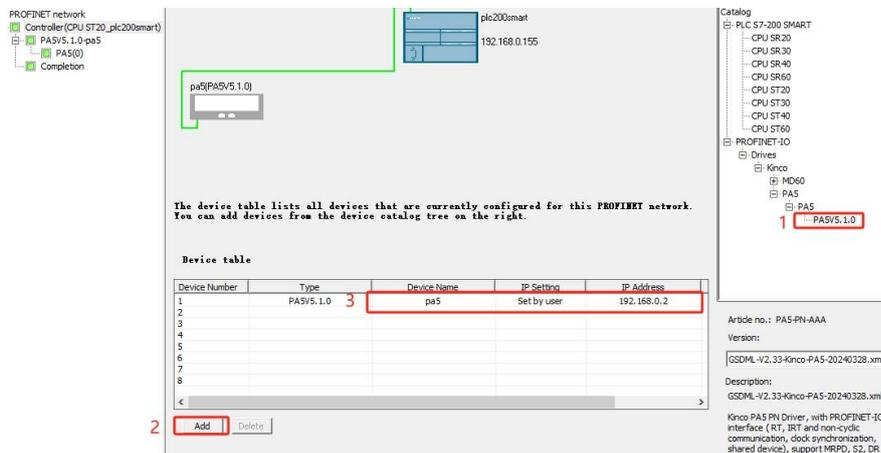
5. Add the PROFIdrive module to the servo, then select and delete the submodule of standard telegram 3 added by default, add the submodule of standard telegram 1, and note down the start address of the I/O data which is needed when calling SINA\_SPEED:
