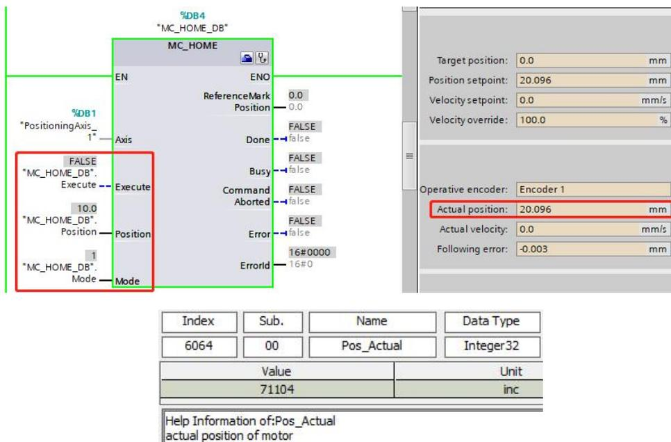
The above figure shows the state before homing, the current position of the axis is 20 mm and the drive actual position [606300] is 71104 DEC.
