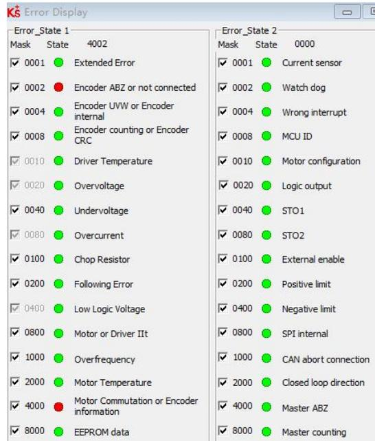
When the drive fault has been eliminated and confirmed, the diagnostics buffer will show that the drive fault event has been cleared:
