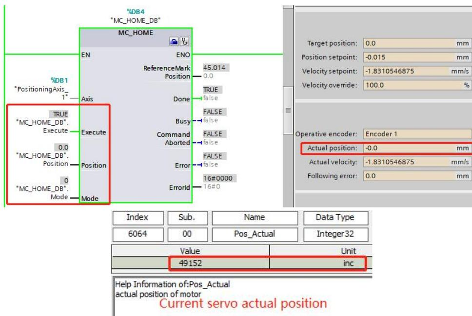
After the homing motion is completed, no matter what position the axis moves to, as long as the PLC is powered off, the actual position data of the axis will be lost and become 0, instead of being converted over with the current encoder value of the drive.
