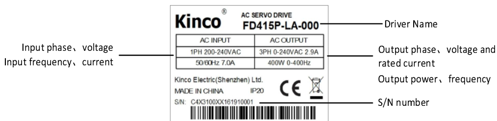
Figure 1-2 Drive nameplate description
