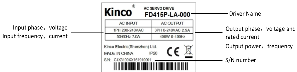
Figure 1-2 Drive nameplate description
